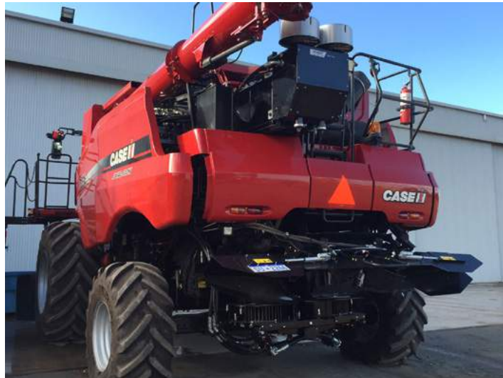
Figure 11: The new integrated Harrington Seed Destructor (iHSD) system is one HWSC method that destroys weed seeds by pulverising the chaff fraction as it leaves the harvester.
