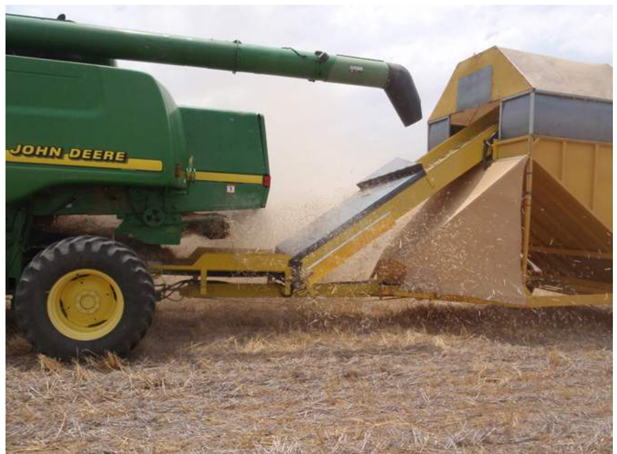
Figure 3: Chaff carts are a practical and proven way to capture a high proportion of weed seeds at harvest.
