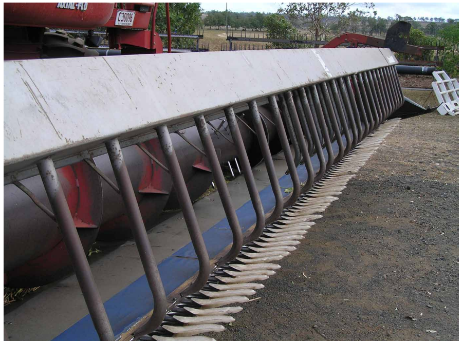
Photo 2: Harvestaire front combined with extension fingers and a blue vibra-mate.
