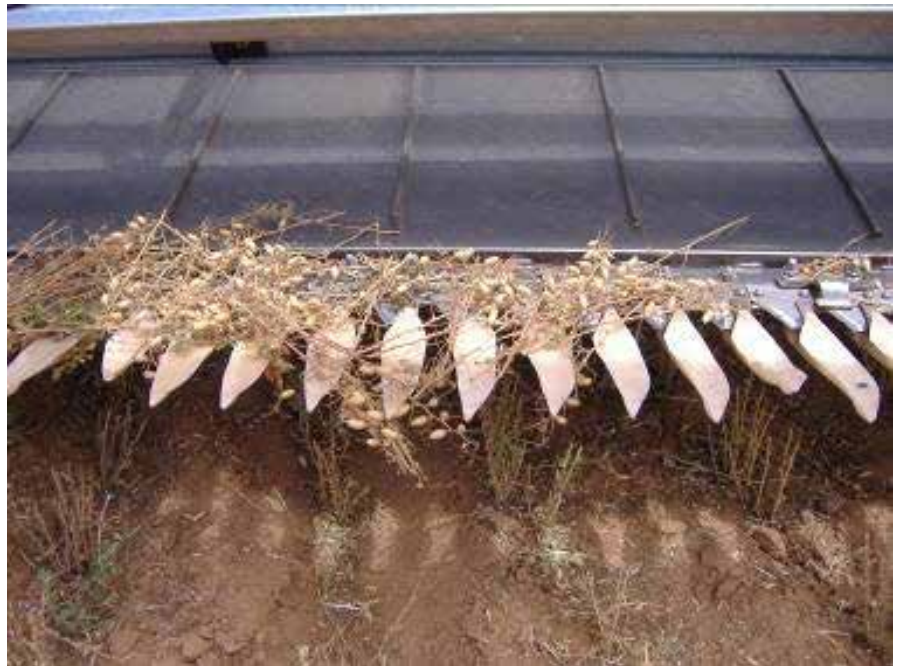
Photo 4: Plastic extension fingers fitted to a draper front.
