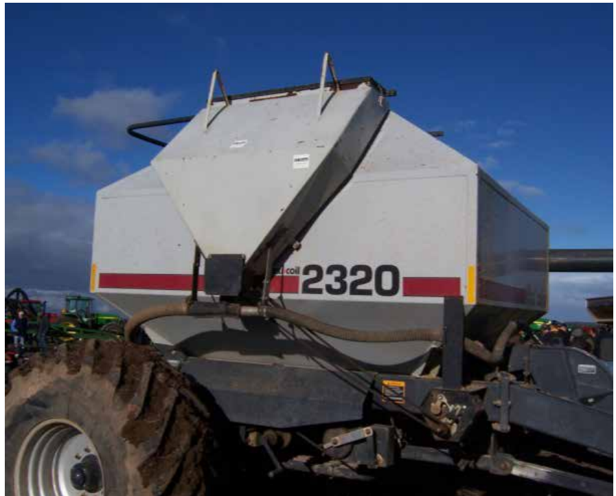
Photo 6: An ‘after-market’ third box fitted to a Flexicoil box to enable application of granular inoculum. Note that granular inoculum cannot be applied mixed with the seed (uneven distribution of seed and/or inoculums occurs). Rhizobia survival is severely jeopardised if granular inoculum is applied mixed with fertiliser.
