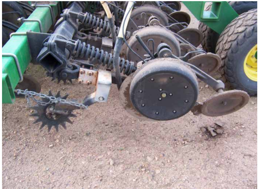
Photo 4: A disc seeder set up with Yetter trash clearing wheels and tubing for liquid injection of inoculum or trace elements during sowing. Note also the closer, covering the seeding slot to act like a press-wheel from the side.
