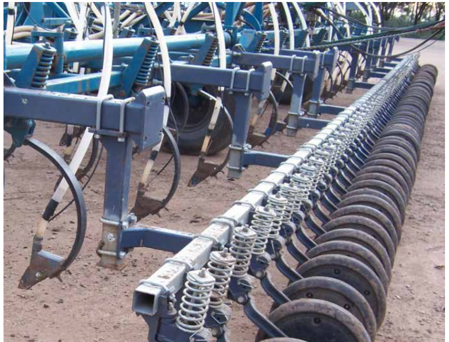
Photo 2: A seeding bar setup with Atom Jet narrow points, gang press wheels and liquid injection for either inoculum or trace element application during sowing.
