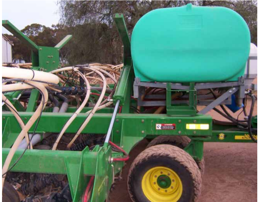
Photo 3: Tanks mounted on the seeding bar for liquid injection of rhizobia or trace elements during seeding. Agitation is required. Note the tubes and manifold. Inoculum must be applied under low pressure only. Some machines have their tanks set up as a separate, trailed tanker.
