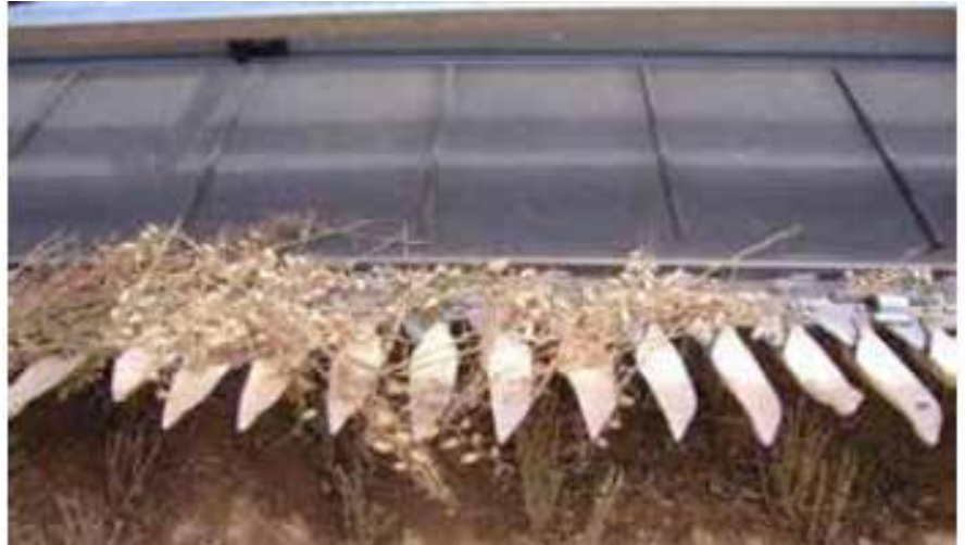
Figure 6: Plastic extension fingers fitted to a draper front.
