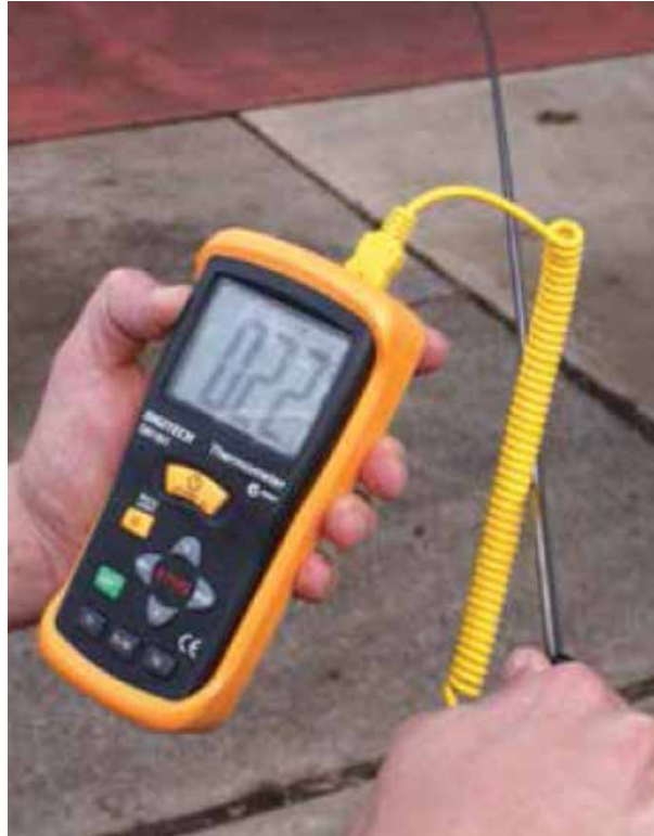
Figure 10: Temperature check: monitor the effectiveness of the cooling process by checking grain temperature with a probe or a thermometer taped to a rod.
