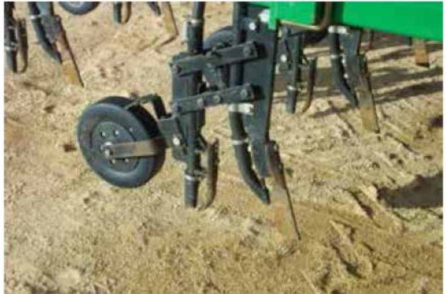
Figure 22: The DBS system parallelogram for uniform seeding depth and deep placement of seed or fertiliser.
