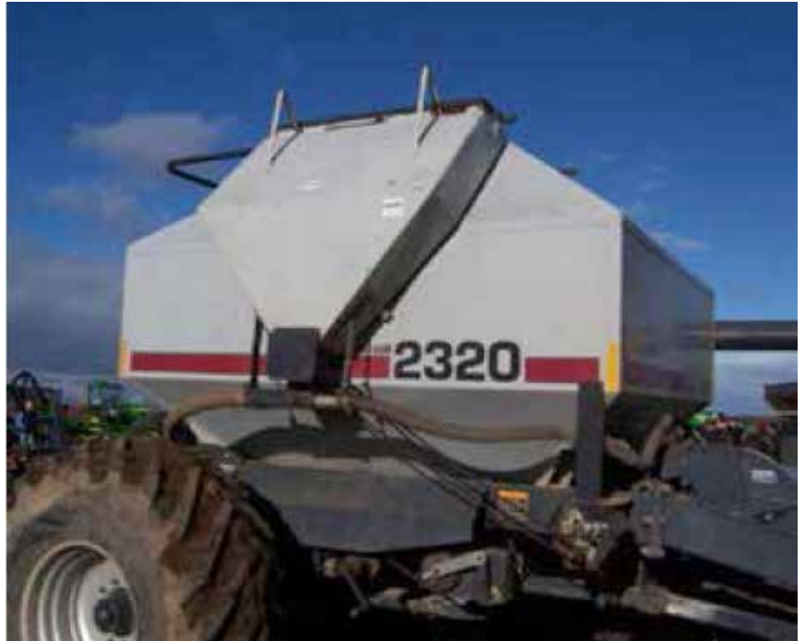
Figure 2: An ‘after-market’ third box fitted to a Flexicoil box to enable application of granular inoculants. Note that granular inoculants cannot be applied mixed with the seed (uneven distribution of seed and/or inoculants occurs). Rhizobial survival is severely jeopardised if granular inoculants are applied mixed with fertiliser.
