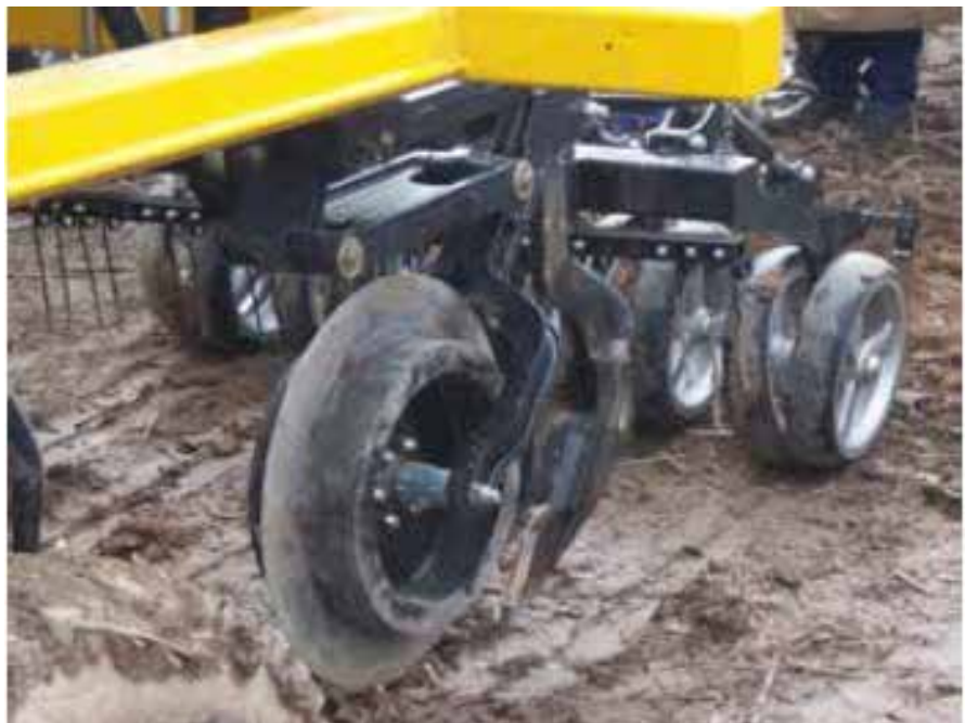
Figure 23: Bio Blade or Cross slot™ disc opener with opening disc and seeding tine, followed by paired press wheels. Note that the seed and fertiliser tube has sharp bends and may not be wide enough to avoid blockages when larger seeded pulses like faba or broad beans are being sown.
