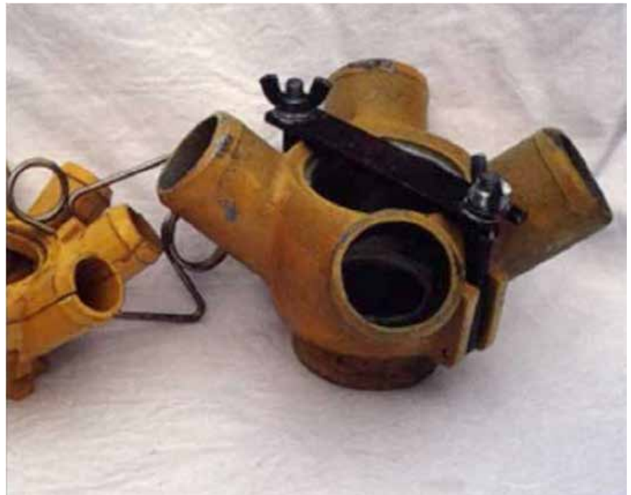
Figure 19: Conversion heads, such as this one for a Connor-Shea airseeder, allow large seeds such as broad beans, faba beans and kabuli chickpeas to be sown with ease.
