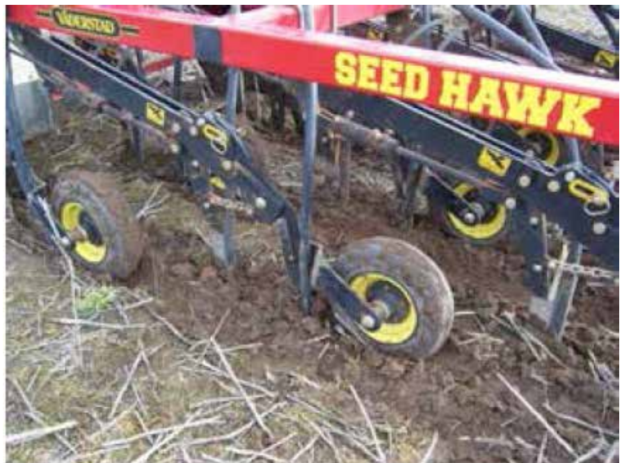
Figure 20: One of several seeding mechanisms for uniform sowing depth using the press wheel for depth control.
